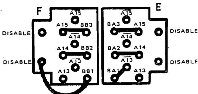
Jumper names: A13, A13, A14, A14, A15, A15 = address lines
