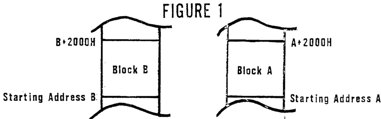
Note that both blocks together occupy 16K of memory. However, there are only 12 sockets for PROMs, and only 1K of RAM on the board, totalling 13K. What happens if the processor addresses memory in the remaining 3K portion? This memory space is NOT necessarily empty. A set of jumpers is provided which in effect specify that the unused 3K, within the 16K, is not on the PROM RAM III board at all, and therefore may be used on other boards.
