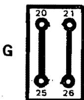
Function: With the board as manufactured, jumper area E is used to address block B, and jumper area F is used to address block A. Furthermore, if the power-on/reset jump feature is used, the jump will take place to the first address in block B.
