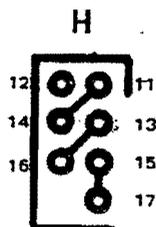
Function: These jumpers allow the user to selectively determine which 3 of 4 1K blocks of memory are returned for use by other boards. These jumpers are selected in conjunction with the RAM memory address jumper in area I, so that together, all 4K of the non-PROM (scratchpad) address space in block B are accounted for. The factory supplied connections complement the factory supplied RAM address jumper, so that the bottom 3K of the scratchpad memory is allocated for use by other boards.
