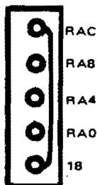
Function: These jumpers allow the user to selectively determine where the RAM addresses are to be located. With the board jumpered as manufactured, the 1K of RAM occupies the top-most 1K of addresses of the 4K scratchpad memory block.
